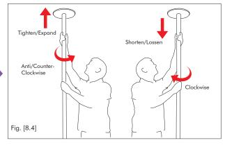
5. POLE ROTATION: Rotating the pole tube from left to the right (Anti/Counter - Clockwise) will Expand/ Tighten the Pole. Rotating the pole tube from right to the left (Clockwise) will Shorten/Loosen the Pole.
