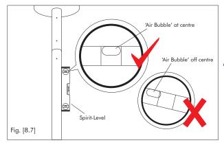
8. Once the Upper Plate is against the ceiling and before it is tightened further, make sure that the pole is vertical. Best way to do this is using a 'spirit-level' (which can be purchased from a local hardware store) or visually align the pole with a door or window frame.
