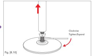
Whilst holding the pole (not allowing the pole tube to rotate) rotate the Tightening/Release Tool Clockwise to tighten the Adjuster.
