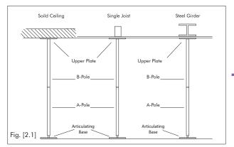
The SPORT POLE should be installed in the most secure location possible, like under a solid ceiling
