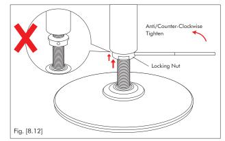
13. Now tighten the Locking Nut until it rises up the Adjuster Rod towards the A-Pole. Insert the adjuster tool into the hole in the locking nut & tighten firmly anti/counter-clockwise. THIS IS THE MOST IMPORTANT PART and ensures that your Adjuster Screw does not become unfastened during use.
