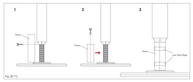
15. If the adjuster is extended, the threads on the adjuster are exposed and could roughen/scratch the dancer's skin. In order to avoid this, a 125mm piece of foam, is included. Fit the foam around the adjuster, by making a vertical slit on the foam, then wrapping this foam around the exposed thread area before use. If the adjuster is less than 125mm cut the foam to the correct size. You may also wish to secure the foam in position by using low-tac tape.
