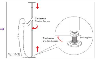
2. To take down the pole, undo the Locking Nut and then unwind the Adjuster Anti/Counter Clockwise until the pole is free from the ceiling. Take care the pole does not fall over. Once the pole has been removed from its position, the Upper Plate & Base Plate can be removed. Lay the pole tubes on the floor and undo the X-JOINTS to disassemble the SPORT.
