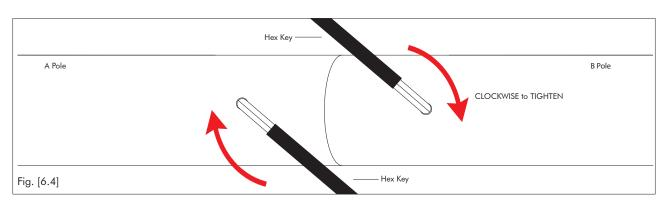
4. It is important to tighten the screws progressively – alternating between the screws, tightening Clockwise. This will ensure the pressure is equalised within the pole tubes.
