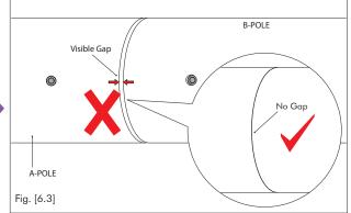
3. Check the tube edges are tight together – then loosely tighten the screw in the A-Pole – now loosely tighten the other tube (B-Pole) – continue to tighten, alternating between the two until no further force could be applied to the screws.
