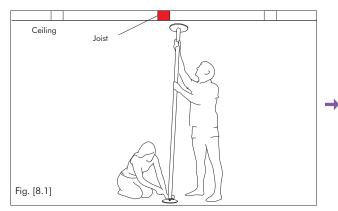
2. With one person holding the base, the other person should slowly and carefully lift the pole, raising it until it is vertical and under the Joist.
