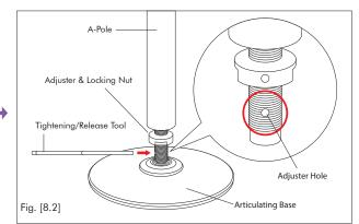
3. Once vertical, the person at the base should insert the tightening/release tool into the hole in the adjuster.
