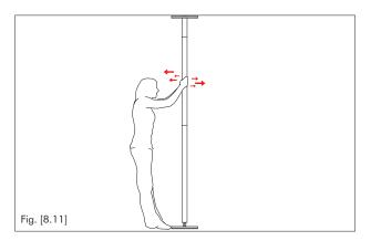
12.Tighten the SPORT pole until good positive pressure is felt and the pole is firmly in place. DO NOT exert too much pressure. Rock/Shake the pole to ensure it does not move from its position.
