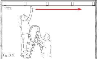
To find a Joist above your ceiling, tap across the ceiling with your knuckle until a solid sound is heard – this will be the Joist. If you keep tapping across the ceiling the sound will become hollow – the space between the Joists.
