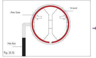
3. The X-Joint features a special mechanism which expands/contracts to lock/loosen the pole tubes together. Please test this prior to assembly.
