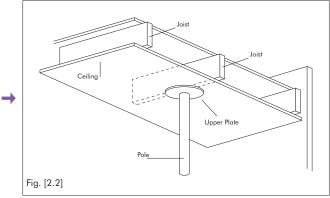
2. Joists are beams of wood that run from wall to wall and support your ceilings. The Upper Plate must be centred on the Joist.
