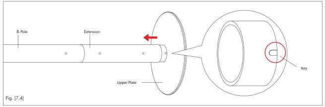
2. As you attach the Upper Plate onto the (B-Pole or last extension used), make sure the 2 x Keys on the Upper Plate locate into the corresponding U Keyway slots [Fig.6.1] on the pole tubes. These Keys stop the pole from rotating.
