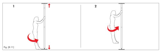
14. Once the pole feels tight and does not move, try practicing a turn with at least one **feet on** the floor. Re-tighten as necessary until there is no movement. Once you are certain that the pole has been installed safely - try a move with your **feet off** the ground.
