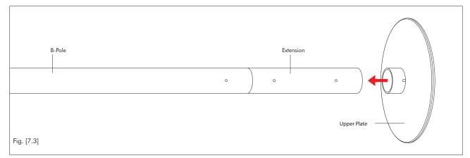
1. Once the A-Pole and B-Pole (and any additional extensions) are connected, insert the Upper Plate into the B-Pole or last extension used.
