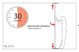
Because the SPORT pole uses pressure to remain in position, over time it could release or become loose. The pole tightness should be checked regularly during use, ideally every 30 mins.
