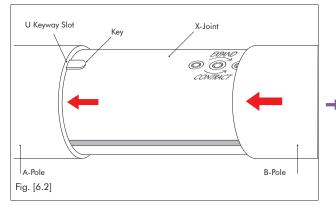
Insert a 200mm X-Joint into the A-Pole (the pole tube with the screw adjuster) ensuring the keys locate into the U Slots and the expansion screws line up with the holes on the pole tubes. Next attach the B-Pole to the A-Pole with the X-Joint ensuring the Keys engage with the U Keyway Slots.
