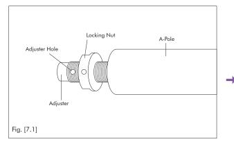
1. Whilst the SPORT pole is on the floor, make sure the locking nut on the A-Pole is loose and you can see the hole in the screw adjuster rod.
