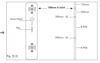
2. The 180mm (7") X-Joint has one half longer than the other & is marked with an arrow (on the shorter end), when used, this must be installed at the top with the arrow pointing upwards.
