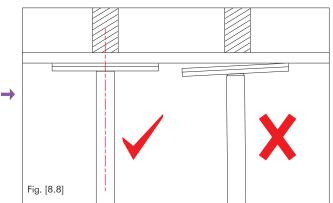
9. It is critical that the Upper Plate is flat against the ceiling/Joist. DO NOT expand the adjuster further until the Upper Plate is flat against the ceiling/Joist. If the Upper Plate is not flat, the plate could rotate, and slip or damage the ceiling.
