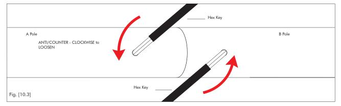
3. To dis-assemble/take apart your pole, lay the pole tubes on the floor and undo the X-Joints to disassemble the SPORT. To undo the X-Joint – turn both Hex Screws **Anti/Counter Clockwise** – undo screws until there is pressure against the key.
