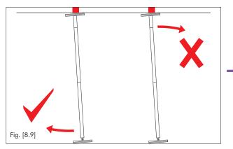
10. If the pole is not vertical, move the base in the required direction. DO NOT move the Upper Plate which must be kept over the centre of the Joist at all times.
